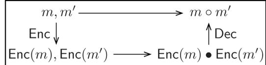
Homomorphism  $\text{Dec}(\text{Enc}(m) \bullet \text{Enc}(m')) = m \circ m'$
