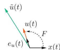
The proposed method cannot be capable for **partial falsification attacks** because the attacks change the length of an input vector and rotate it. The authors will extend the proposed method so that it cancels scalar multiplication and rotation.
