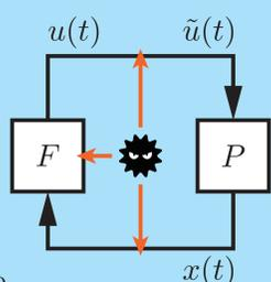
By using malleability, adversaries can conduct pole-assignment attacks even if control systems are encrypted. This type of attacks is called **malleability-based pole-assignment attacks**.
