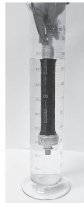
Fig. 4 Measuring the volume of PAM with a Messzyliner
